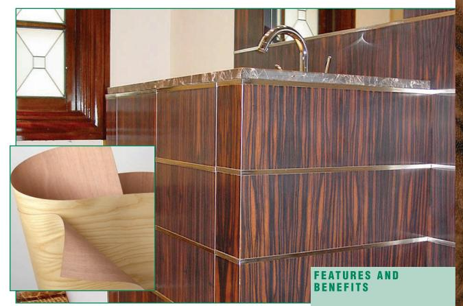
FormWood 2-Ply veneer has a perpendicular face-to-back construction utilizing a thin acrylic membrane to provide protection against bubbling, glue seepage and telegraphing.
