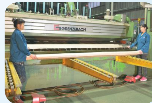
Vertical Veneer Slicing
