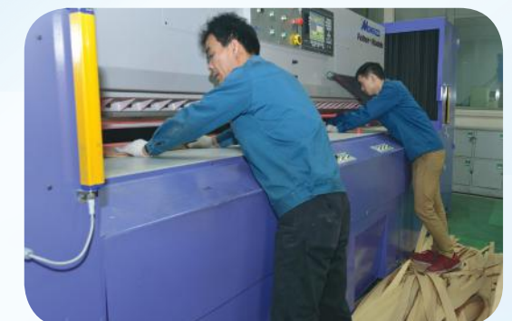
Double Blade Veneer Cutting
